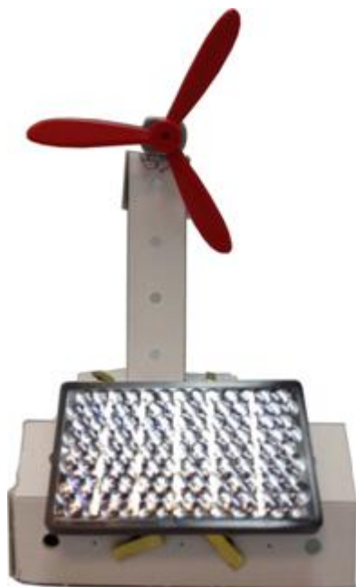
Figure 3. Model of a photovoltaic energy converter
